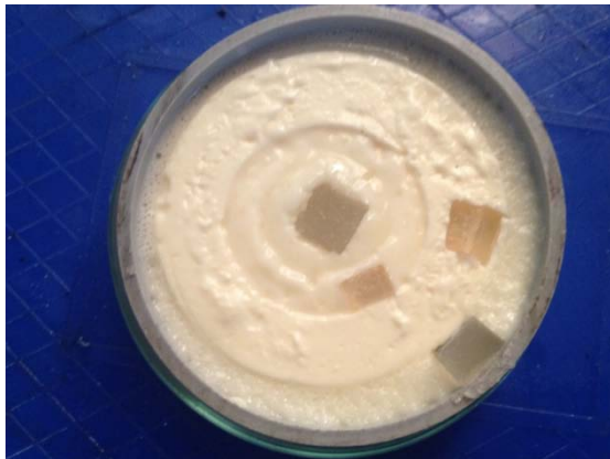
Fig. 5: Tumor embedded in each layer of heterogenous phantom.
